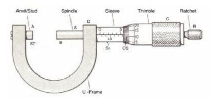
**Zero error:** zero of the head scale coincides with the pitch scale axis.
