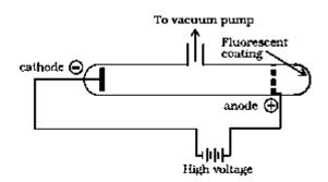
This was caused by the rays that originated from the cathode hence called cathode rays.
