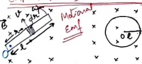
Consider a bar of length, l rotating with angular speed,  $\omega$  about a pivot at one end, O. Consider a segment of the bar of length,  $dr$ , whose velocity is  $v$ .
