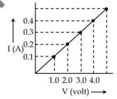
**85.** The current flowing through a conductor and the potential difference across its two ends is as per readings of the ammeter and the voltmeter shown below.
