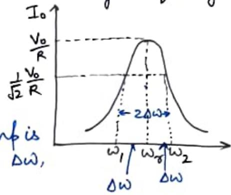
$\omega_1$  &  $\omega_2$ : Values of  $\omega$  for which the current amp is  $1/\sqrt{2}$  times its max<sup>m</sup> value. Smaller the value of  $\Delta\omega$ , the sharper or narrower is the resonance.
