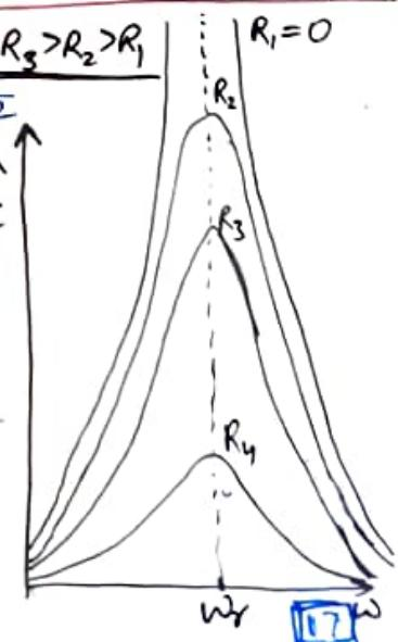
The sharpness of resonance of a circuit is described by its quality factor,  $Q$  ( $Q$ -factor)
