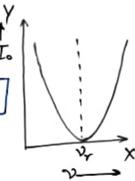
\* In parallel L-C circuit, At Resonance, Circuit doesn't allow any current to flow thro' it. ∴ Impedance must be max<sup>m</sup>.
