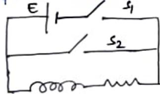
at time  $t$ , let  $I$  be the current flowing in the circuit. Current doesn't decay instantly b'coz induced current by  $L$  will support the decay of current & oppose the change in current.
