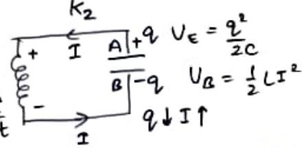
(iii) A stage will reach, which capacitor is totally discharged ( $q=0$ ), current reaches its max<sup>m</sup> value,  $I_0$
