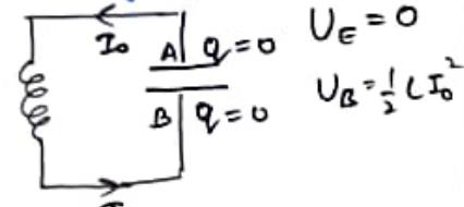
(iv) As the capacitor is totally discharged & there is no flow of current, current tends to decrease (to I, say), e.m.f induced in the coil would oppose the decrease in I
