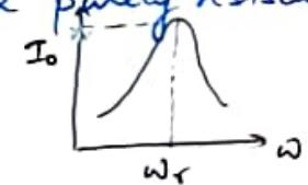
\* The freq. ( $\omega_r$ ) of the applied voltage for which the current in RLC circuit becomes max<sup>m</sup> is called the resonant frequency.
