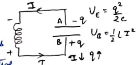
(v) Soon plate B will acquire +ve charge & plate A will attain equal -ve charge. The capacitor gets charged again but with opposite polarity.
