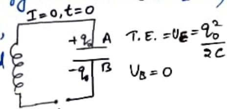
(ii) On closing the key,  $K_2$ , the plates A & B are connected with each other. The electrons from plate B move towards A, which constitutes  $C = \frac{Q}{d}$  current in opposite direction. As induced emf opposes the change in  $I$ .  $\therefore I$  will inc slowly not instantaneous &  $q \downarrow$
