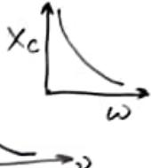
$$X_C \text{ Vs } V \text{ :- } X_C = \frac{1}{\omega C} = \frac{1}{2\pi f C} ; X_C \propto \frac{1}{\omega}, X_C \propto \frac{1}{f}$$
