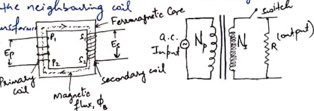
$P_1, P_2 \rightarrow$  Primary coil,  $S_1, S_2 \rightarrow$  Secondary coil. A source of alternating e.m.f is connected to pri coil & a load resistance, R is connected to secondary coil.
