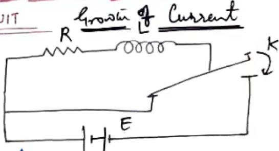
On pressing  $K$ , the battery is connected. Current grows in the L-R circuit. Due to self-induction, an induced emf is set up across  $L$ . By Lenz's law, Induced emf opposes the growth of current.
