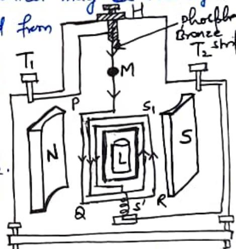
\* S' (Hair spring) :- provides passage of current for the coil, keeps the coil in posn, generates the restoring torque on the twisted couple.
