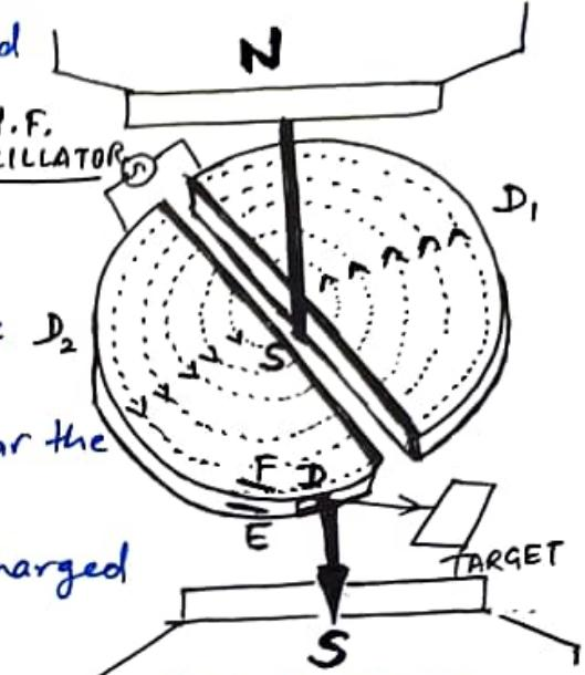
Working and Theory :- When a positive charge is emitted from the source, S, At any instant, suppose  $D_1$  is at -ve potential &  $D_2$  is at +ve potential. Therefore, the positively charged ion produced at S, will be accelerated towards  $D_1$ . On reaching inside  $D_1$ , the ion will be in a field free space. Hence, it moves with a const. velocity in  $D_1$  (say  $v$ ). But due to mag. field ( $B$ ), the ion will describe a circular path of radius,  $r$  in  $D_1$ .
