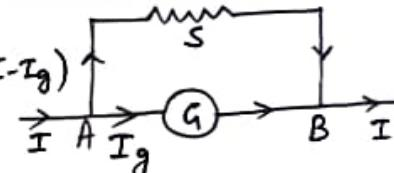
The effective Resist.  $R_p$  of Ammeter (i.e., shunted galvanometer):
