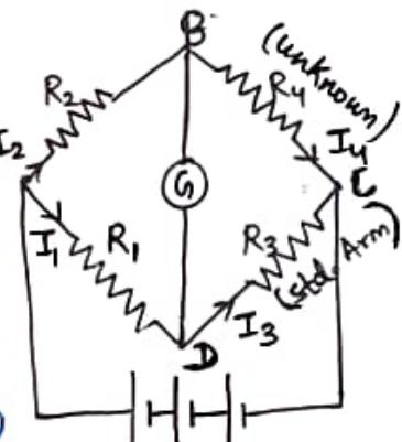
METER BRIDGE :- It's the special case of wheatstone Bridge & simplest form of wheatstone Bridge. It's useful for comparing Resistances more accurately.
