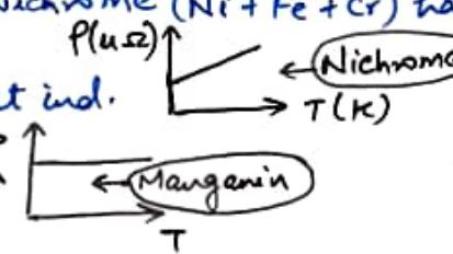
• The  $\rho$  of Manganin is almost ind. of temperature. This is why wire bound std resistors are made of manganin.
