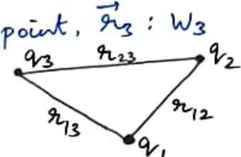
$$\therefore \text{Total W.D.} = U = 0 + \frac{k q_1 q_2}{r_{12}} + \left( \frac{k q_1 q_3}{r_{13}} + \frac{k q_2 q_3}{r_{23}} \right)$$
