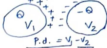
Electric field in the region b/w the conductors,  $E \propto Q$  (Coulomb's law)
