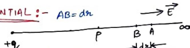
P.d. ( $dV$ ) b/w B & A = W.D. in moving unit positive test charge from A to B.
