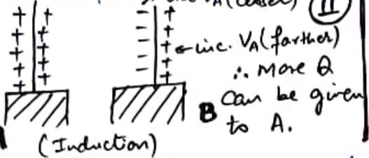
Consider another insulated metal plate B held near plate A. By Induction,  $-Q$  is produced on the nearer face of B & an equal  $+Q$  develops on the farther face of B.
