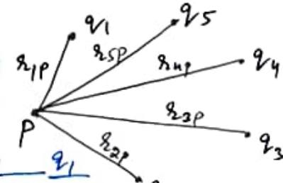
The Potential,  $V_1$ , at  $P$  due to the charge,  $q_1 = \frac{1}{4\pi\epsilon_0} \frac{q_1}{r_{1P}}$
