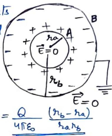
As, outer sphere B is earthed, therefore, its pot.,  $V_B = 0$
