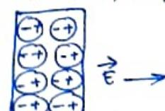
When a non-polar molecule is placed in an electric field, the centres of +ve & -ve charges get displaced & the molecule is then said to have been polarized. The induced dipole moment is prop. to the applied  $\vec{E}$  & it is almost independent of temperature. Further, the induced dipole is parallel to the electric field right at the time of its creation.
