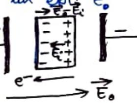
As applied & induced electric field inside the cond. are eq. & opp.  $\therefore$  Net Electric field in the interior of cond. is zero.
