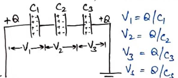
{ Such an arrangement is used where the working voltage is high & a single capacitor can't sustain it }
