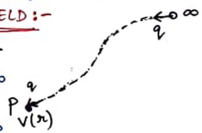
$$\therefore \text{E.P.E. of the charge, } q \text{ (at } r\text{)} ; \underline{U(r) = -W.D. = -q \int_{\infty}^r \vec{E} \cdot d\vec{r} = qV(r)}$$
