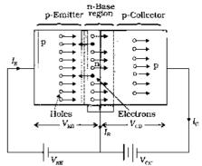
The emitter-base of the **p-n-p transistor** is forward-biased by connecting it to the positive pole of emitter-base battery  $V_{\text{EE}}$  and the collector is reverse-biased by connecting it to the negative pole of the collector-base battery  $V_{\text{CC}}$ .
