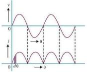
As we are getting output in the positive half as well as the negative half of the AC input cycle, the rectifier is called a full-wave rectifier. Obviously, this is a more efficient circuit for getting rectified voltage or current than a **half-wave rectifier**.
