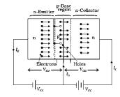
The remaining electrons cross into the collector region and enter the positive terminal of the battery  $V_{\text{CC}}$  connected to the collector.
