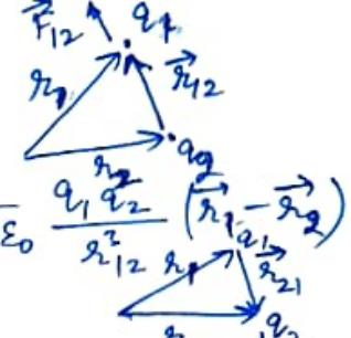
The Force on charge,  $q_2$  due to charge,  $q_1$  :  $\vec{F}_{21}$
