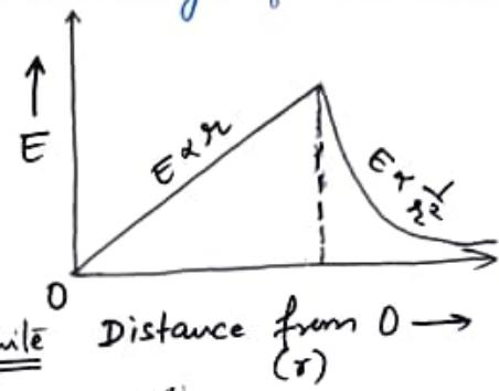
(iv) Electric Field Intensity due to a thin infinite plane sheet of charge :-
